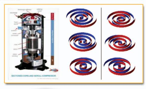
In a scroll compressor refrigerant is compressed by two offset spiral disks that are nested together. The upper disk is stationary while the lower disk moves in orbital fashion. The orbiting action of the lower disk inside the stationary disk creates sealed spaces of varying volume. Refrigerant is sucked in through inlet ports at the perimeter of the scroll.
