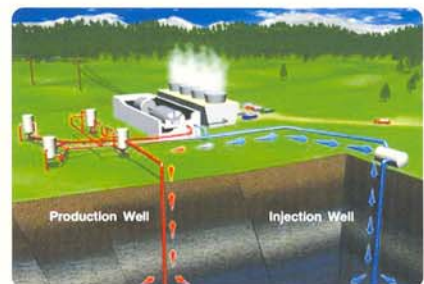
Large temperature differential system using local heating
